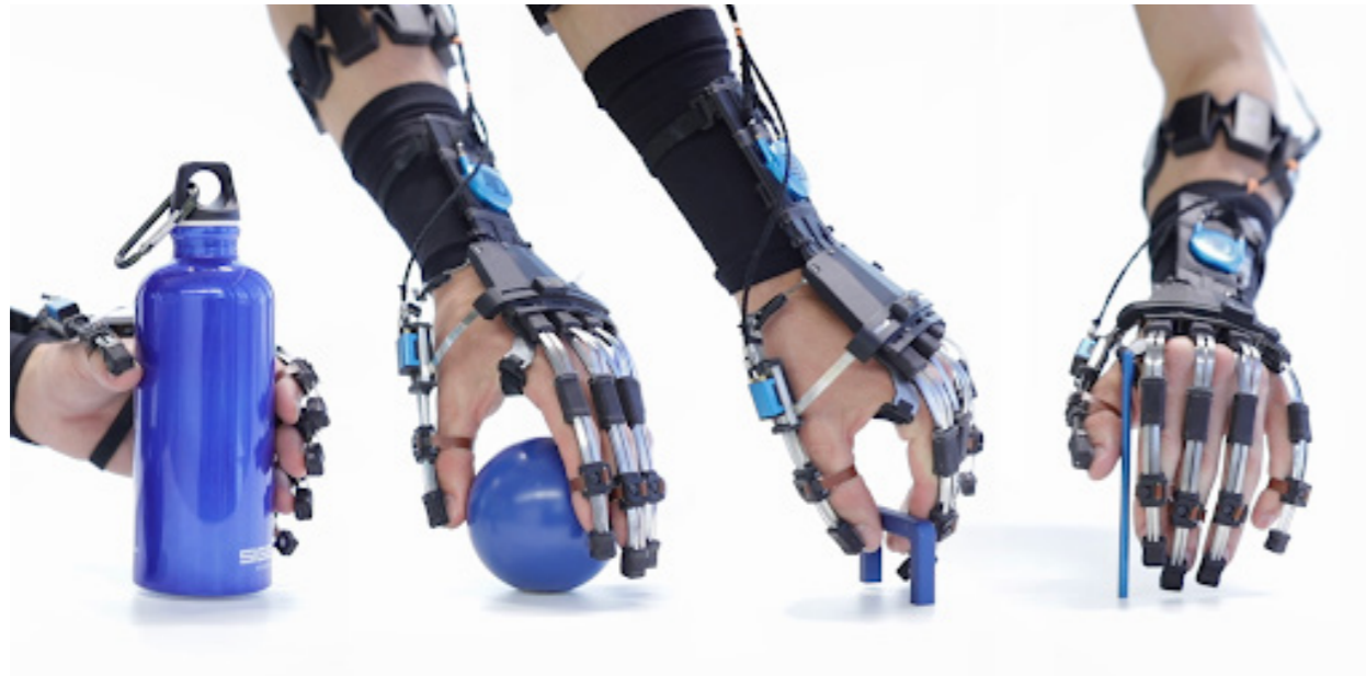
The Relab tenoex allows users to change the force range and closing speed, select between two grasp types, and configure the control system/intention detection strategies. Image credit: RELAB ETHZ
